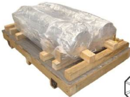
4 Layer Vacuum using VCI and Nylon + Aluminum.
